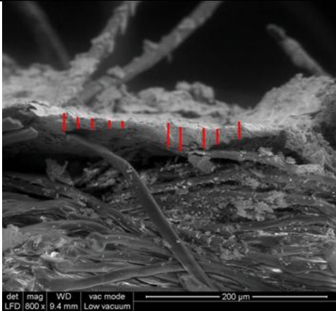
Fig. 3: Measured thickness of the 100 mm Ag coating
